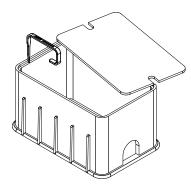
CLEAN LID GROOVE -Remove dirt, roots, debris
